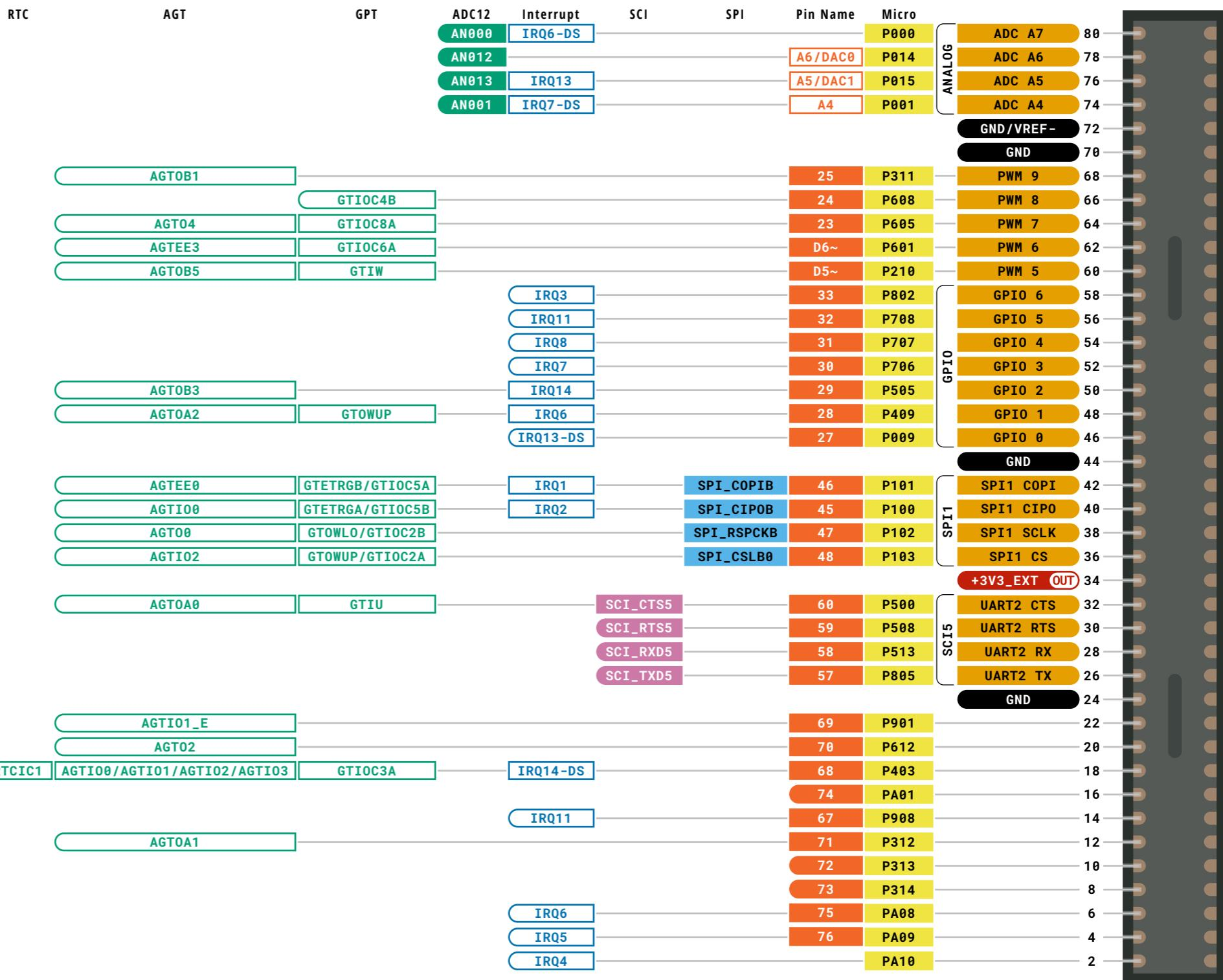
Using the numbers in the "pin name" column on the Arduino IDE, you can control the corresponding pins
