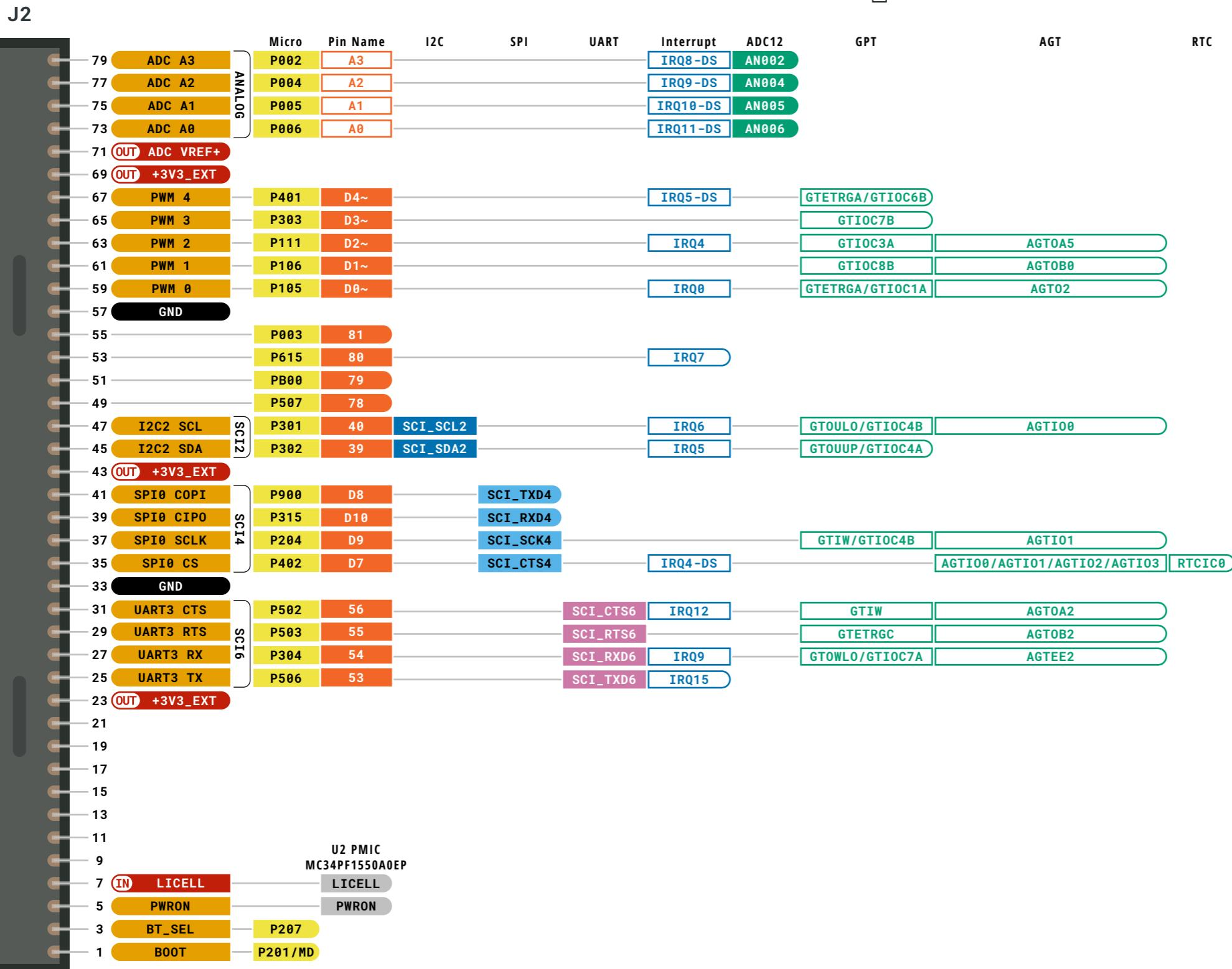
Using the numbers in the "pin name" column on the Arduino IDE, you can control the corresponding pins
